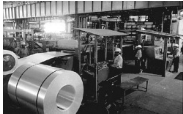
Fig. 6.6: Strip coating mill at smelter of NALCO
