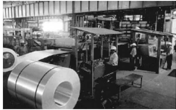
Fig. 6.6: Strip coating mill at smelter of NALCO
